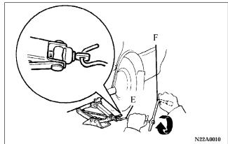
8. Insert the bar (E) into the wheel nut wrench (F). Then attach the end of the bar to the jack end, as shown in the illustration.
